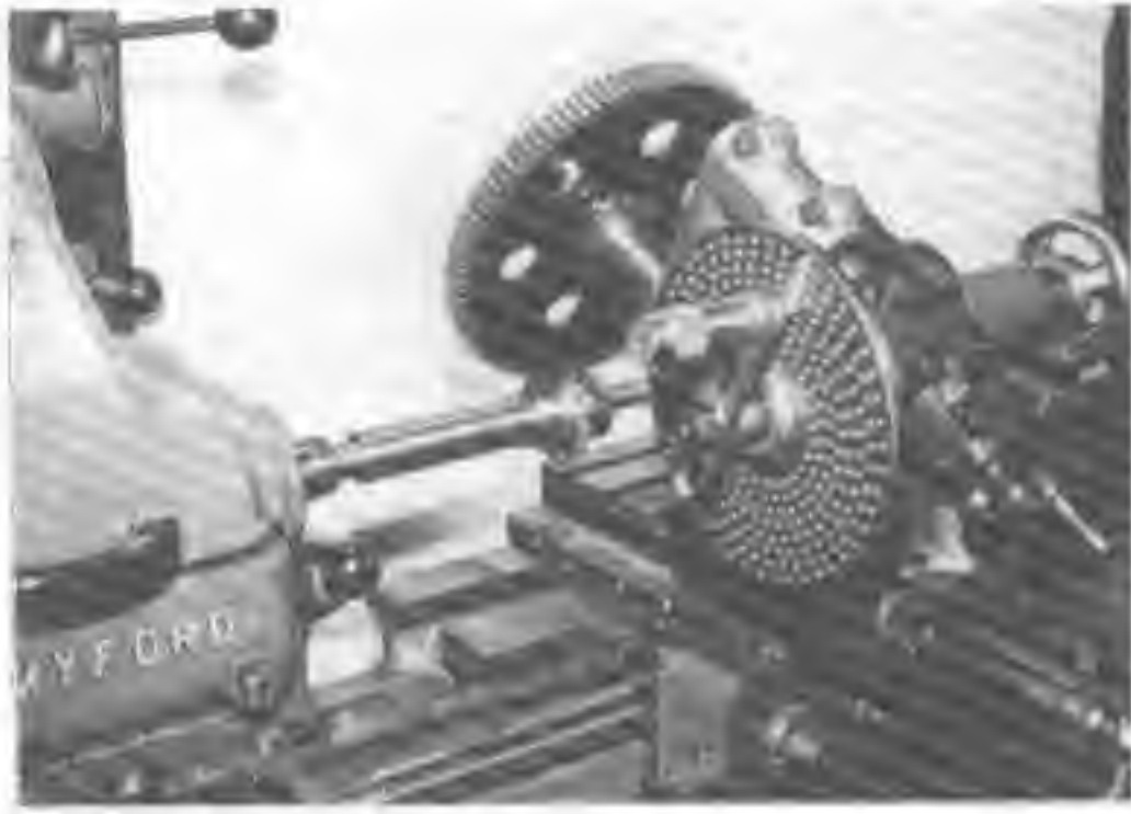
Fig. 62 This large gear precludes the use of a tail support. A short arbor is used to obtain maximum rigidity.
